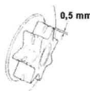
Check for cracks and for excessive wear interfering with the chain drive. If the wear is considerable, replace it with new one. Never fit a new chain on a worn sprocket, or a worn chain on a new sprocket.
