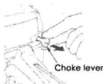
*Note: When restarting immediately after stopping the engine, set the choke knob in the first-stage position (choke open and throttle lever in the starting position)*
