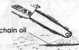
The chain oil flow can be changed by inserting a screwdriver in the hole on bottom of the clutch side. Adjust according to your work continuous.
