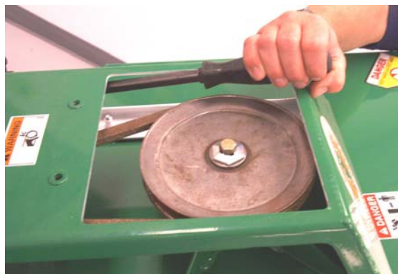
Adjusting Blade Drive Belt Tension
