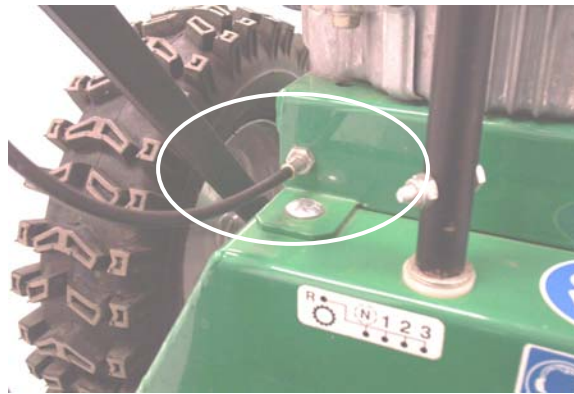
Blade Cable Adjustment
