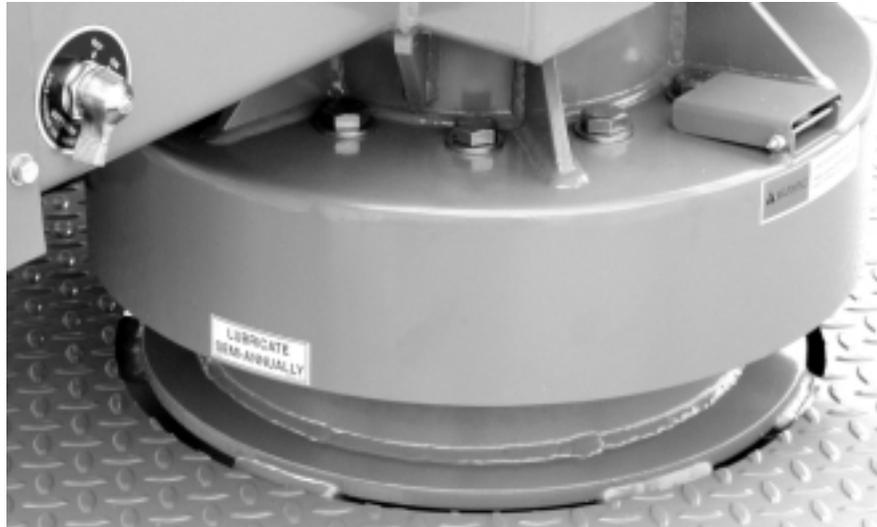
**Figure 4-3. Lubricate Semi-Annually**
