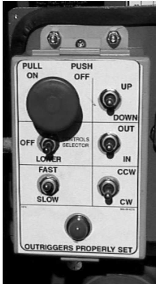
Figure 3-2. Lower Control Panel (DC Model)
