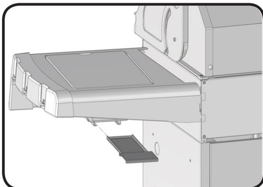
**WARNING!** The Infrared side burner is supplied with a drip pan which holds only a minimal amount of grease. To prevent grease fires, the pan must be cleaned after each use.
