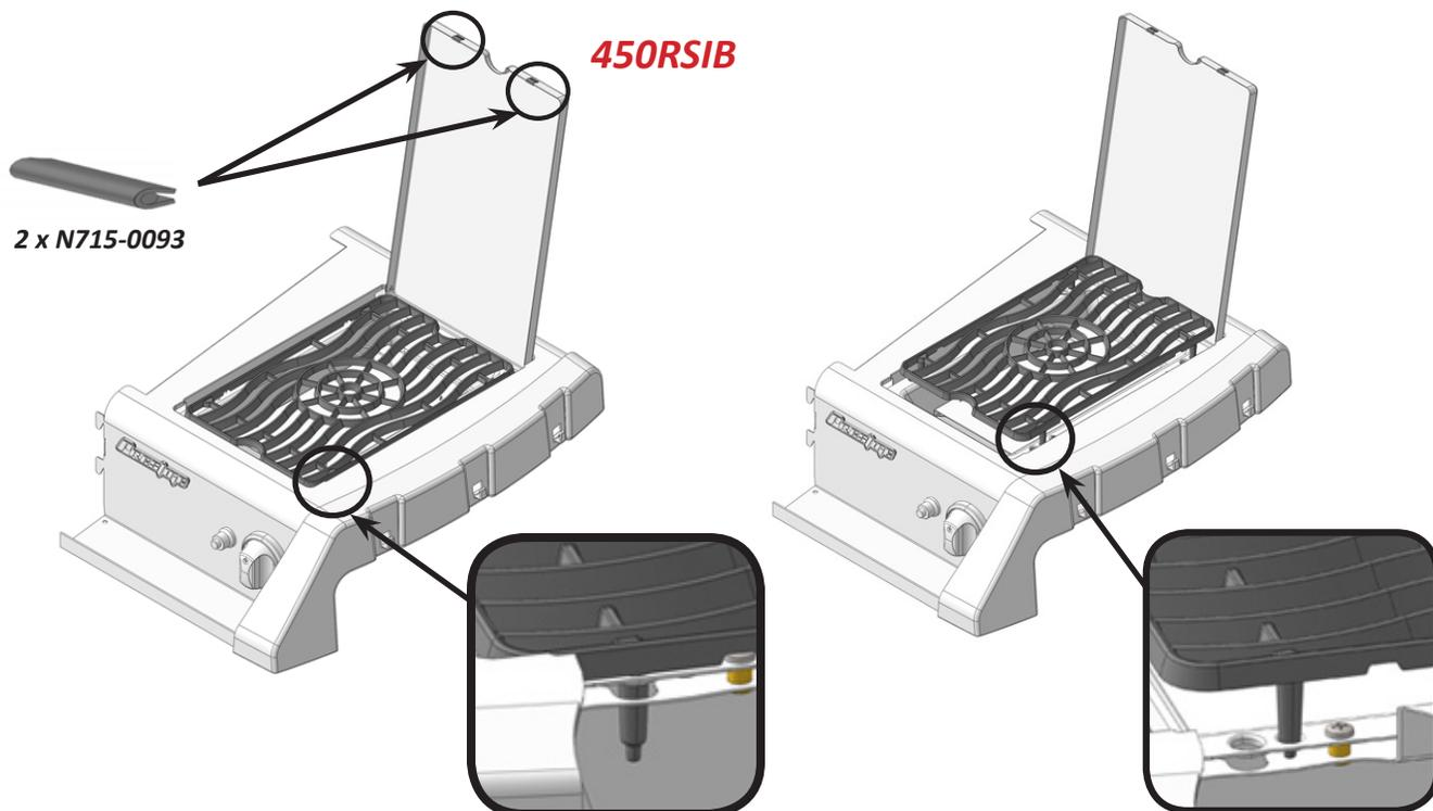
**Cooking Grid Placement:** The cooking grid can be placed at two different heights. The lower height is for use with pots or pans. The higher position is to be used when searing meats. Ensure the burner is off and the grid is cool to the touch before changing between the two heights. The grid must be at the lower height in order to close the lid.
