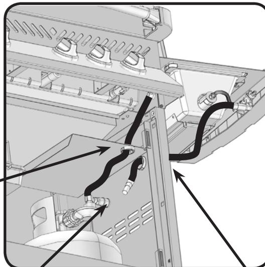
Plug the side burner hose into the quick disconnect.
