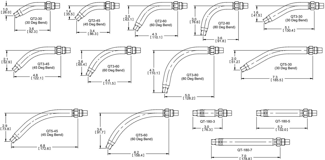
Notes: Dimensions in brackets are in millimeters. Diffuser thread size: 1/4-18 NPT "Bernard Special".
