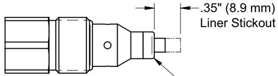
Adjust liner stickout dimension by threading brass liner lock deeper onto plastic material. Turn clockwise for approximately 8 turns.
