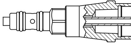
When using optional Jump Liner in neck, trim the plastic liner from SGA kit flush with the front edge of the brass adapter as shown.
