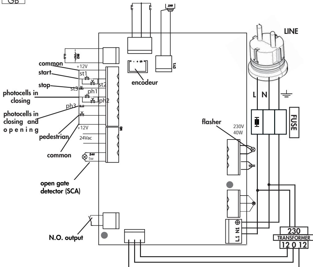
**The current feed line (230V L,N,GND) towards the automated device must be protected by a magnetometric switch or by a pair of 5A fuses.** A differential switch is recommended but not indispensable if it is already found at the top of the system.
