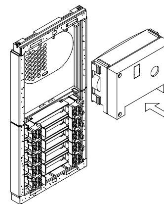
Insert the sound module in the grille module. For a proper assembly, align the light push button and the microphone rubber of the sound module with its corresponding holes in the grille module.
