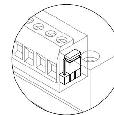
EL551 sound modules for systems with several access doors have a jumper placed on the right side of the terminal connector. This jumper allows to select between two different electronic call types, allowing the user to distinguish which door panel is calling.
