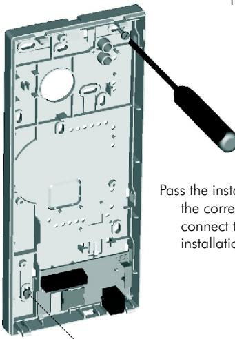
Pass the installation wires through the corresponding hole and connect them as shown on the installation diagrams.
