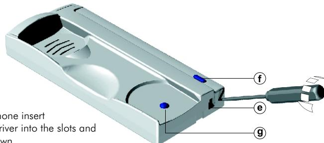
To open the telephone insert a plain screwdriver into the slots and rotate it as shown.
