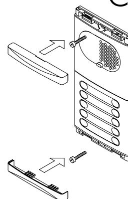
Fix the door panel by using the supplied screws.
