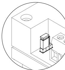
EL555 sound modules for systems with one access door have a jumper placed on the left side of the terminal connector. This jumper allows to select between two different call types: electronic call (factory default) or buzzer call.
