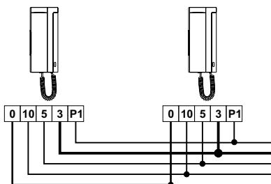
The maximum number of telephones placed in the same apartment is three. For each telephone placed in parallel the section corresponding to the call wire must be doubled.
