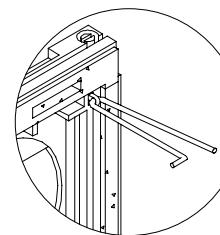
Select a direction to open the door panel; this selection should ease the door panel wiring.
