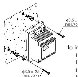
To install the transformer directly on the wall, insert the fixing flanges. Drill two holes of Ø6mm. and insert the wallplugs. Fix the transformer with the specified screws.
