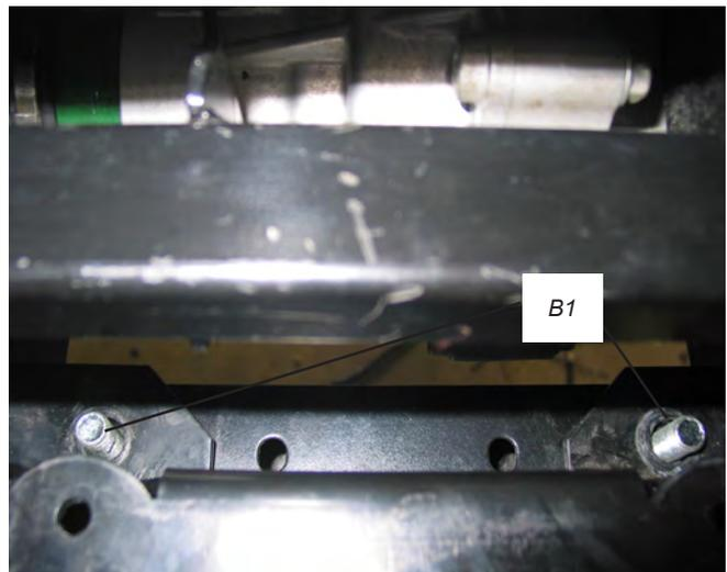
Figure 8 Install fasteners
