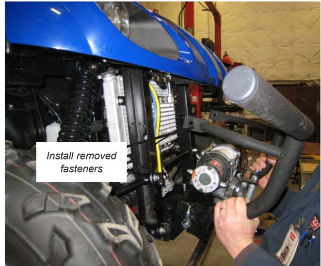
Figure 7 Place Bumper on vehicle
