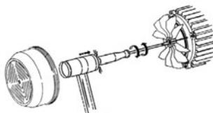
Check that the direction of motor rotation corresponds with that indicated on the specification plate (the fan should rotate in a CLOCKWISE DIRECTION, when viewed from the rear of the motor. If the motor is three-phase and it is observed that it is rotating in the opposite direction, then two of the supply phases should be inverted at the protection panel).
