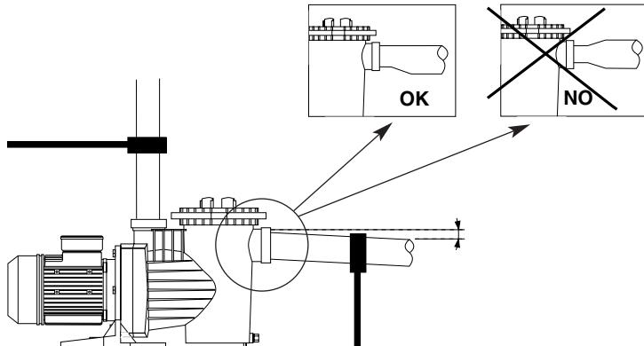
It is very important that both the suction and impulsion piping are independently supported and correctly fixed in place so that the pump does not have to support their weight nor the vibration produced by the water flow through them. In a situation where a long length of impulsion piping is used, we recommend the installation of a check valve to prevent the water hammer produced by the return of the water causing any damage when the pump stops.
