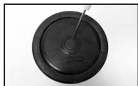
2. Under the cap there are four holes. Align one of the holes with one of the two flanges that are holding the cover on. Then slide the screwdriver through that hole and on top of the flange. Now pry the screwdriver up, thus putting pressure on the flange and pull the cover up with the other hand. The cover will pop off with ease for easy access to the impact.
