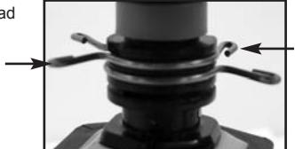
3. Now spread the 2 adjusting trip collars by pushing on one of the tabs to the desired Part Circle degree. Make sure that the reversal trip mechanism, which is mounted to the adjustment tab, is NOT in the horizontal position (flipped up) and is in the vertical position (flipped down) between the 2 adjusting trip collars in order to reverse properly in the Part Circle mode.
