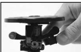
**NOTE:** When switching nozzles, make sure to note the location of the arm spring and switch the spring arm if required. The Pro Impact is shipped with the spring arm in the A position. Only the #6, #7, and #7 low angle nozzles require the spring to be changed the B position. In the B position there is less tension on the spring, which allows for better tripping of the impact on those light flow nozzles.
