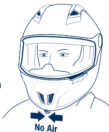
Switch to centre – ventilation disabled
