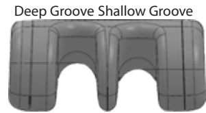
End View of Cable Slide Fig. 2
