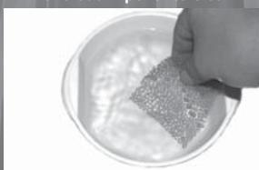
Remove filter from housing and clean in water
