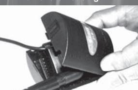
Then connect the second half of the housing from the bottom first, then close together.
