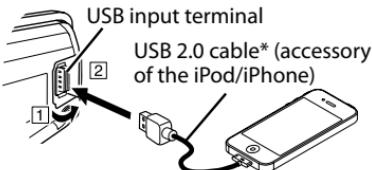
The source changes to "USB" → "USB-IPOD" and playback starts (depending on the status of the connected device).
