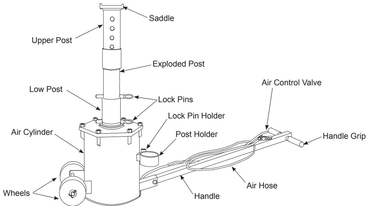
Figure 1 - Air Jack/Support Stand Components
