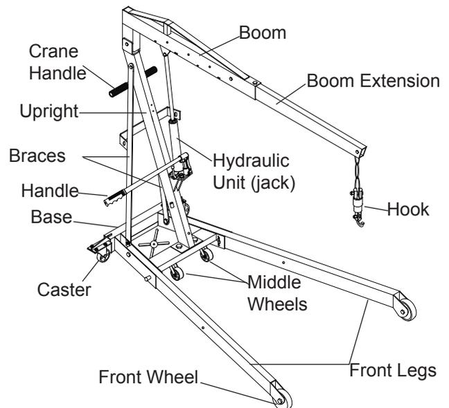
Figure 2- Model Atd-7485 Components
