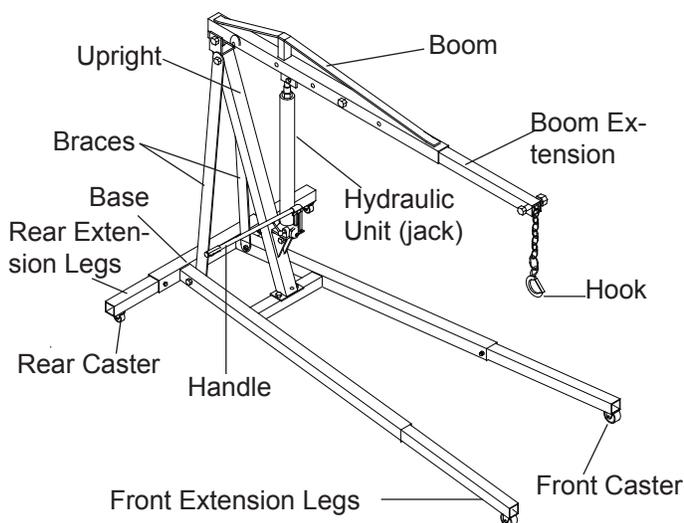
Figure 1- Model Atd-7484 Components
