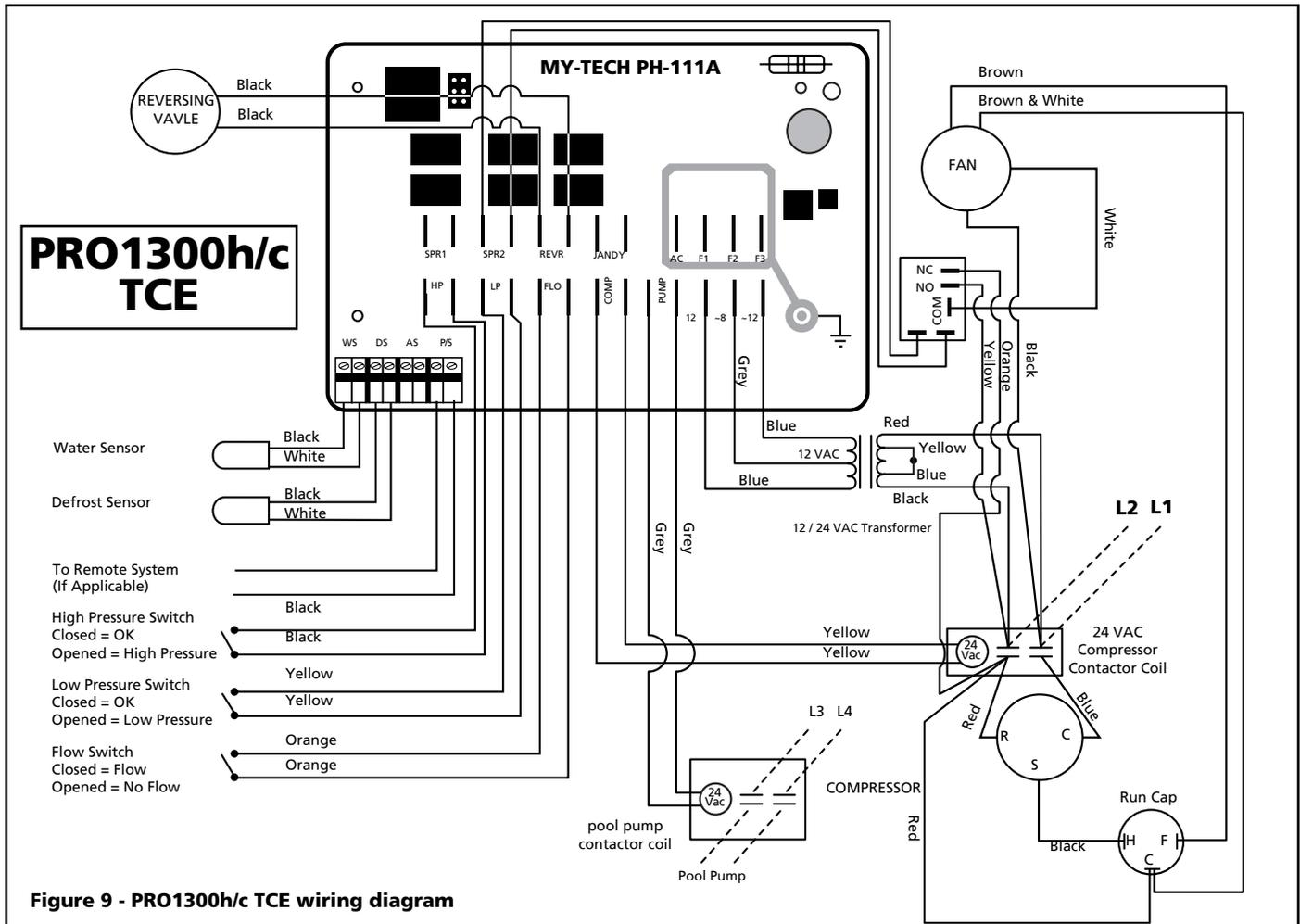
Figure 9 - PRO1300h/c TCE wiring diagram
