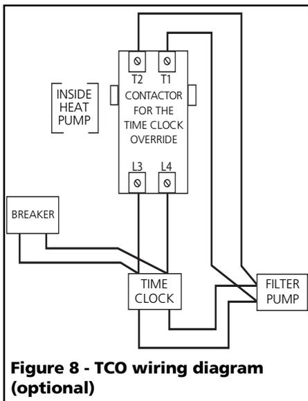
**Figure 8 - TCO wiring diagram (optional)**
