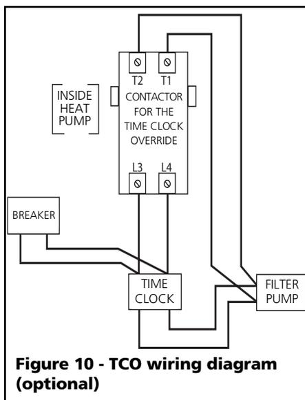
**Figure 10 - TCO wiring diagram (optional)**
