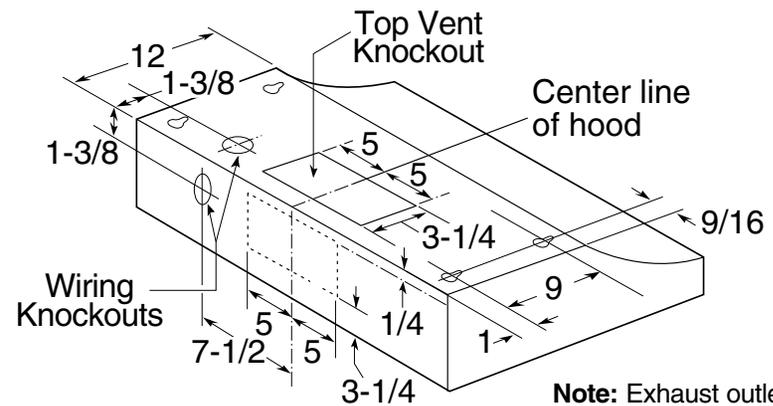
**Note:** Exhaust outlet connects to 3-1/4" x 10" rectangular duct. Vent top or rear. Includes rectangular damper.
