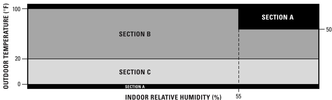
**SECTION A:** Controller will not ventilate due to temperature extremes
