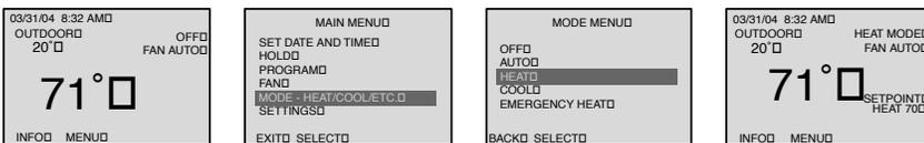
2. Adjust the thermostat set point to a temperature higher than the displayed room temperature, using the Up button, so that a Heat call is initiated. Again, consult your thermostat Owner's Manual for details on how to do this properly.
