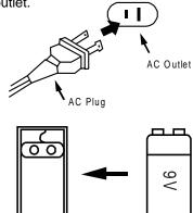
Be sure to check the condition of the battery periodically by disconnecting the AC cord and connecting it again 2 or 3 minutes later. The preset times should continue operating. If the clock resets to "12:00" on the Clock Display, it indicates the battery is dead or not connected properly.
