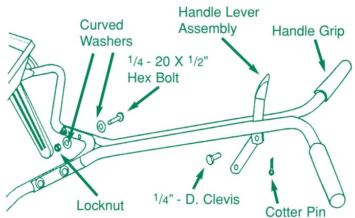
**4** Stand spreader upright on wheels. Attach upper handle assembly to handle brace (make sure handle is positioned as shown) using four 1/4-20 X 1 1/2" hex bolts, eight curved washers, and four locknuts. Tighten securely. Install handle grips onto upper handle. Slide handle lever assembly between handle brackets and secure with 1/4 diameter clevis and cotter pin. Make sure lever pivots freely.
