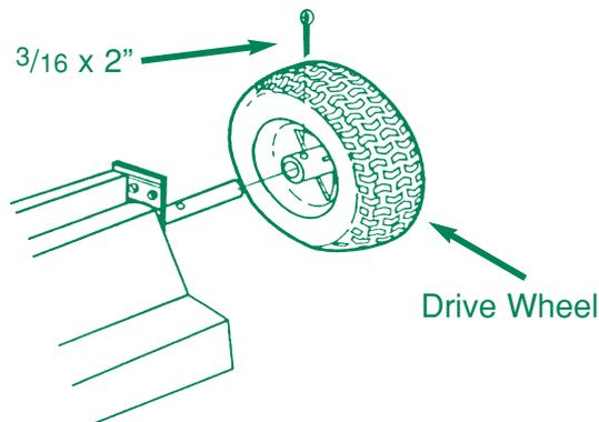
**2** Slide wheels onto each end of axle with the longer portion of the wheel facing the hopper. Secure wheels with 3/16 dia. x 2" cotter pins.
