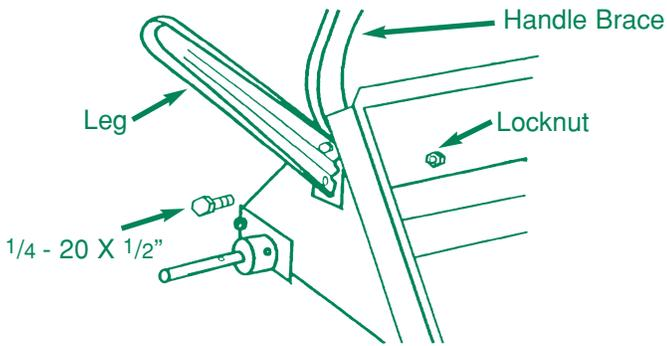
**1** Remove spreader and components from carton. Place hopper on its front panel, insert two 1/4-20 X 1/2" hex head bolts through the leg; flattened end of handle brace and holes in hopper as shown. Install hex locknuts but do not tighten. Repeat on opposite side.
