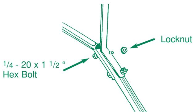
**3** Install control tube between the control tube braces and secure with two 1/4-20 X 1 1/2" hex bolt and locknuts.
