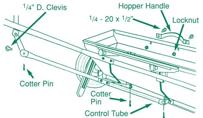
**5** Slide the ends of the control tube braces over the studs on the shutoff bar brackets; secure with cotter pins. Attach opposite end of control tube to the handle lever using 1/4 diameter clevis and cotter pin. Make sure handle lever operates freely. **Tighten all Nuts left loose in Step #1.** Install hopper handle on front of spreader using two 1/4-20 X 1/2" hex bolts and locknuts.
