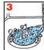
Cleaning cycle is complete when cleaning foam entirely disappears from disposer and you hear a swish of water (approx. 3-4 min.). Rinse remaining foam from sink and turn off disposer.
