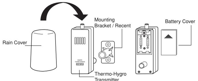
should be permanently mounted only after the signal reception has been verified.
