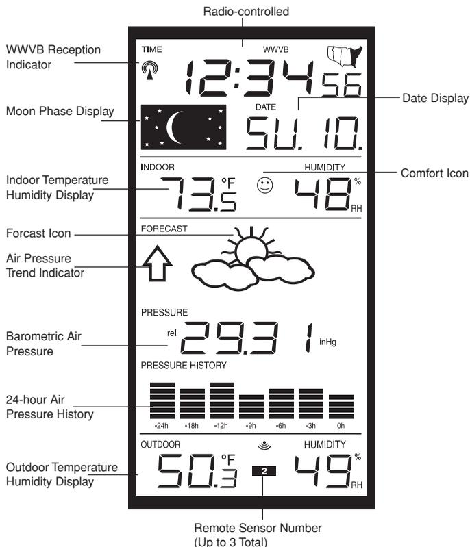
B. There are many different modes the indoor weather station can be set to. The LCD shown is the normal operating mode, and your actual data shown will be different based on your local settings and conditions.
