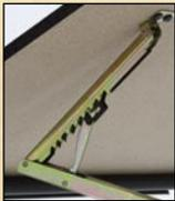
Tilt mechanism for MiniMaster II
