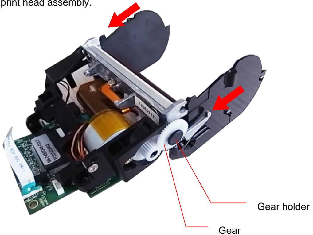
4. Reassemble the parts in the reverse procedures.
