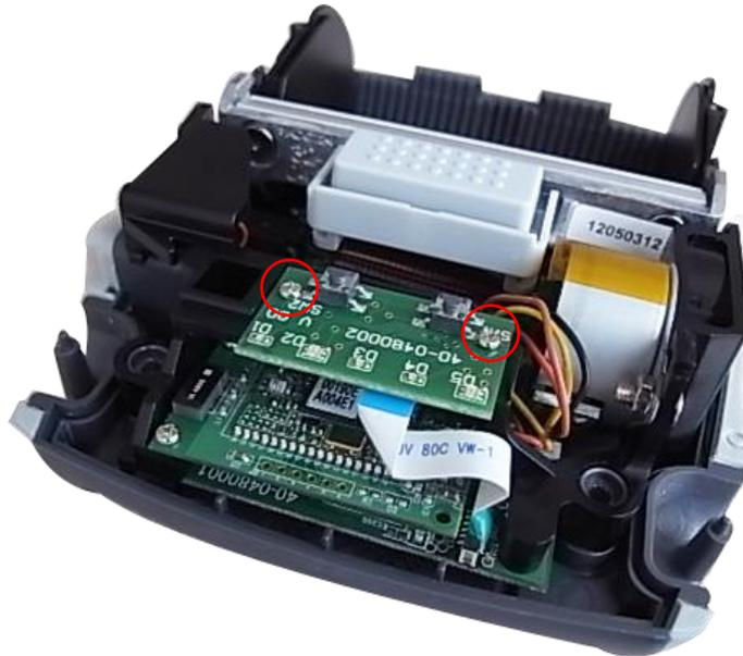
3. Loosen the connector lock then disconnect the flat cable from the keys control board. Remove/Replace the keys control board.
