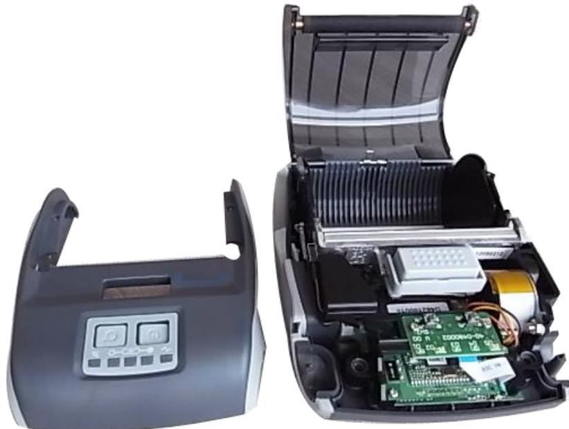
3. Use a tool to remove the shaft. Remove/Replace the media cover. (including the platen roller ass'y)
