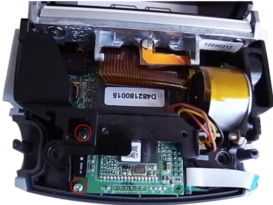
3. Disconnect the connector on the board.
