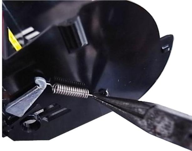
3. Take the gear holder and the gear, and push the print head holder on the each side to remove the print head assembly.
