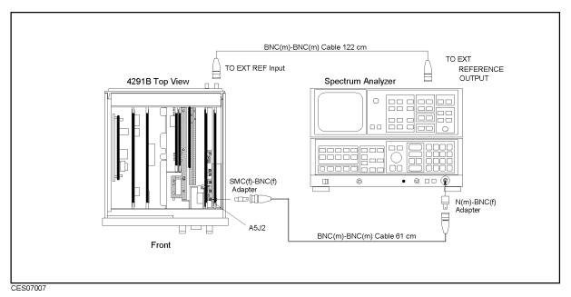
Figure 7-7. STEP OSC Test Setup
