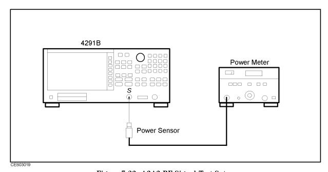
Figure 7-23. A3A3 RF Signal Test Setup
