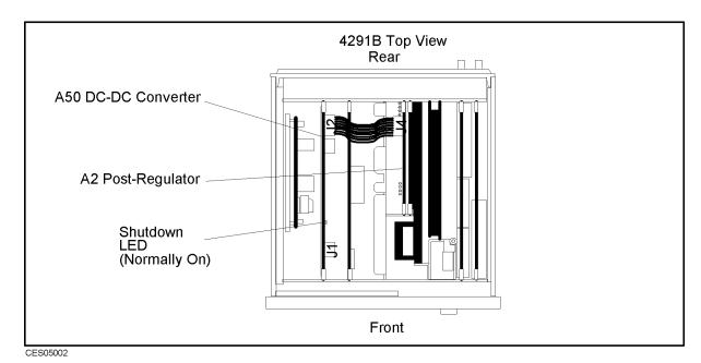
Figure 5-2. A50 SHUTDOWN LED Location
