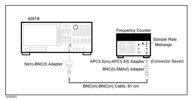
Figure 2-1. Frequency Accuracy Test Setup
