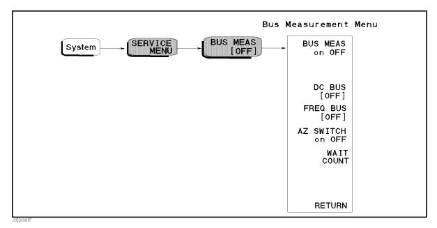
Figure 10-6. Bus Measurement Menu
