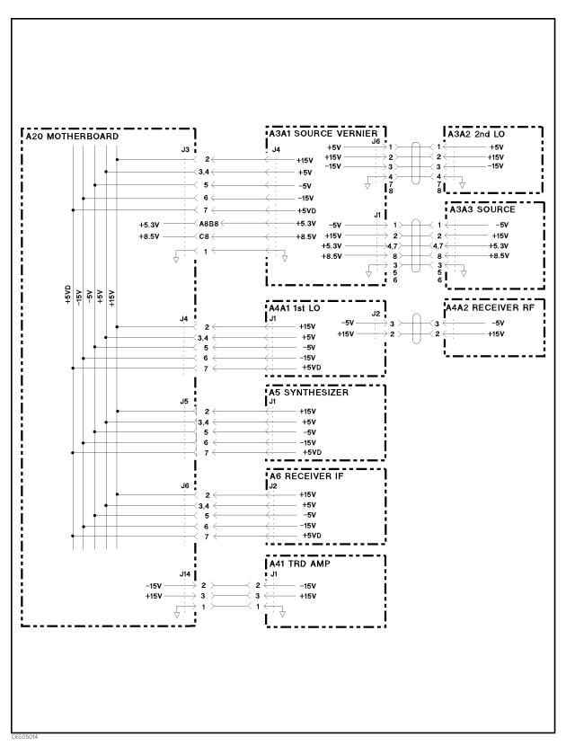
Figure 5-14. Power Supply Block Diagram 3
