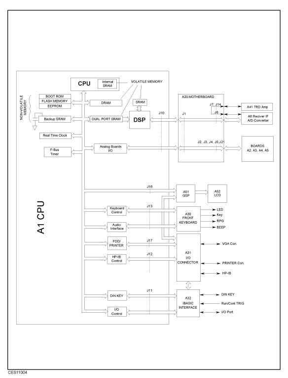
Figure 11-4. Digital Control Group, Simplified Block Diagram
