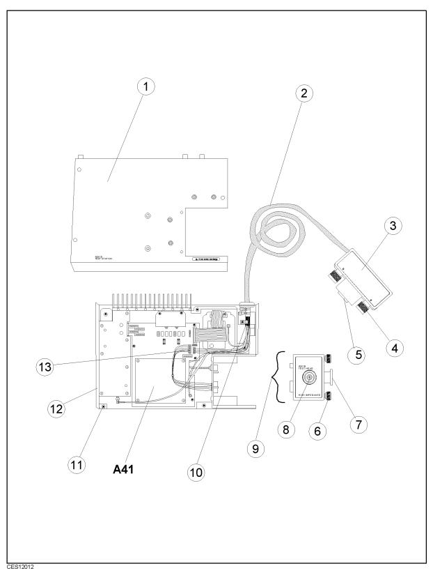
Figure 12-17. Test Station and Test Head Parts
