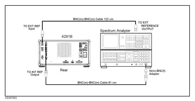
Figure 7-2. INT REF Test Setup
