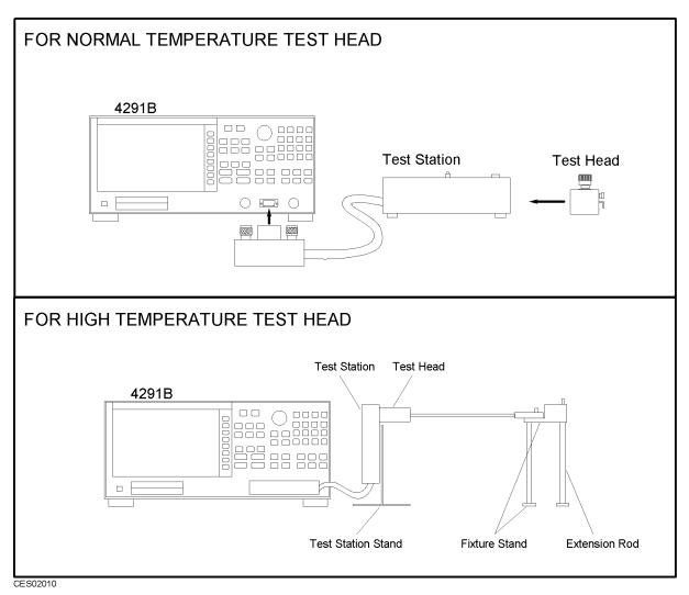
Figure 2-3. Measurement Accuracy Test Setup
