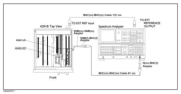
Figure 7-17. 21.42 MHz Signal Test Setup
