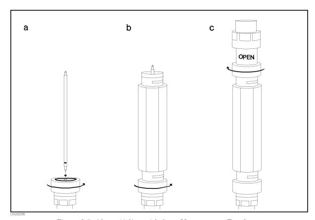
Figure 2-5. 10 cm Airline with Open Measurement Test Setup
