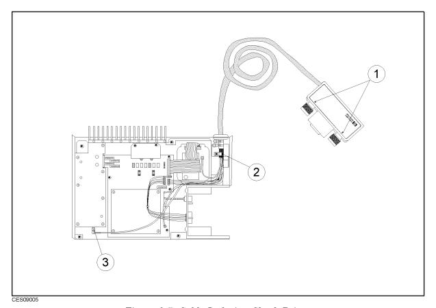
Figure 9-5. Cable Isolation Check Points
