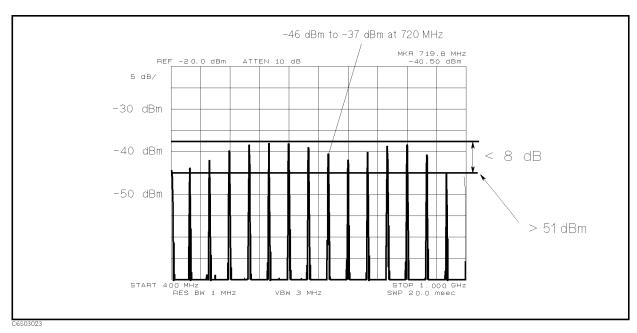
Figure 3-8. Comb Generator Output
