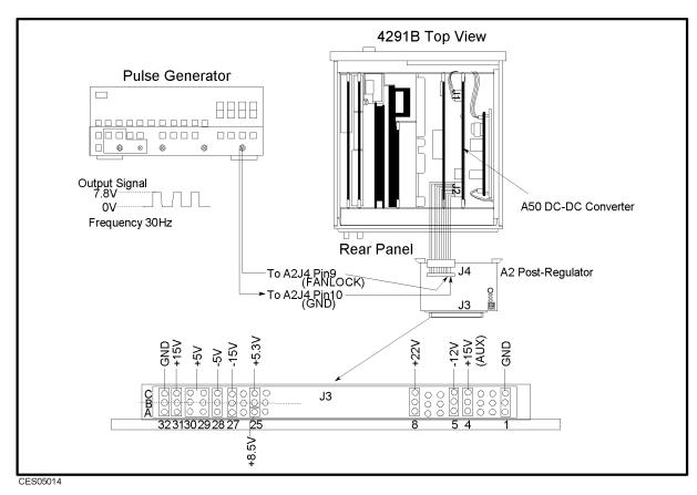
Figure 5-11. A2 Output Voltage Measurement Setup
