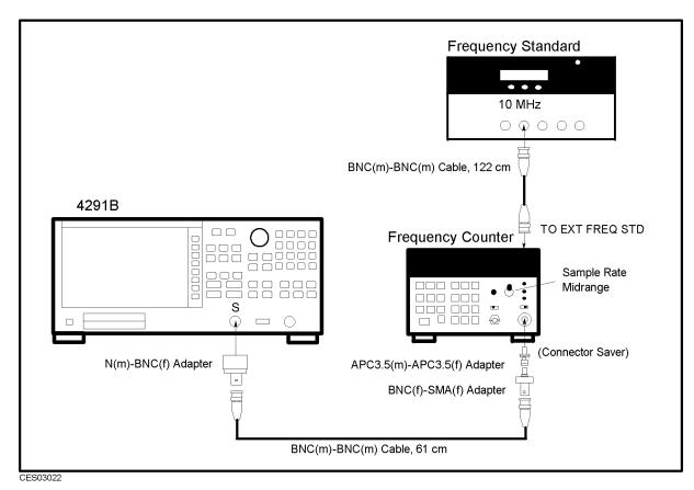
Figure 3-21. 10 MHz Reference Oscillator Frequency Adjustment Setup
