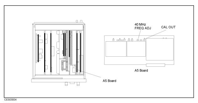
Figure 3-3. 40 MHz Reference Oscillator Frequency Adjustment Location
