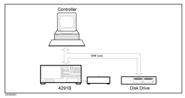
Figure 3-1. Updating Correction Constants Setup
