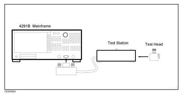
Figure 4-4. Transducer Test Setup
