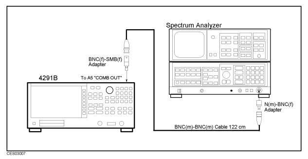
Figure 3-6. Comb Generator Adjustment Setup
