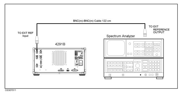
Figure 7-11. EXT REF Test Setup
