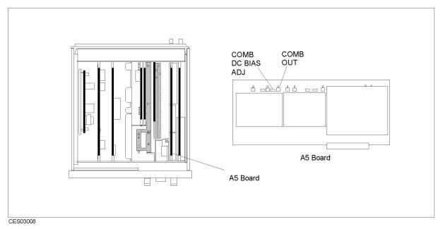
Figure 3-7. Comb Generator Adjustment Location
