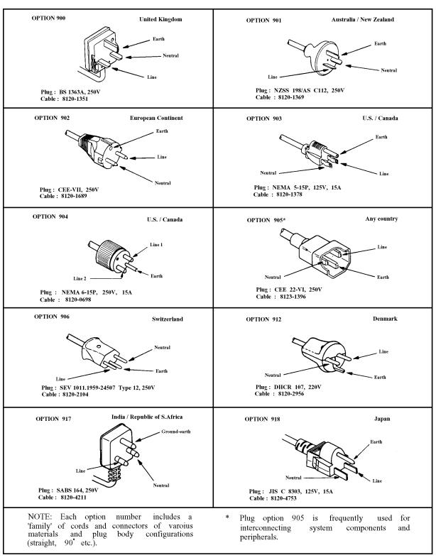
Figure B-1. Power Cable Supplied
