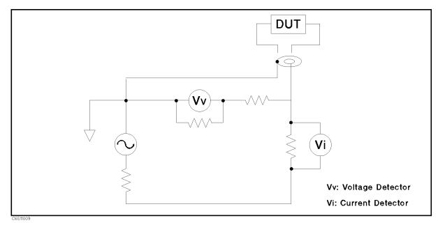
Figure 11-9. Low Impedance Measurement Block Diagram
