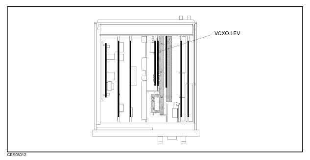
Figure 3-11. Source VCXO Adjustment Location
