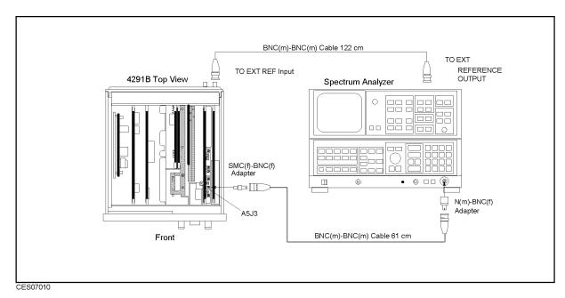
Figure 7-10. 520 MHz Signal Test Setup
