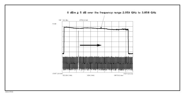
Figure 7-14. Typical 1st LO OSC Signal (Single Mode) at A4A1J3
