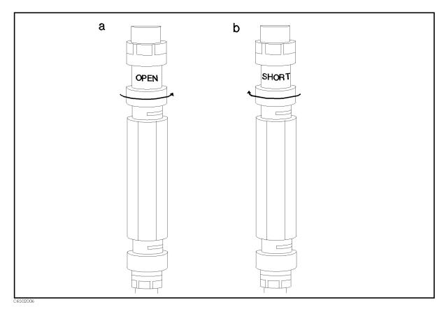
Figure 2-6. 10 cm Airline with Short Measurement Test Setup
