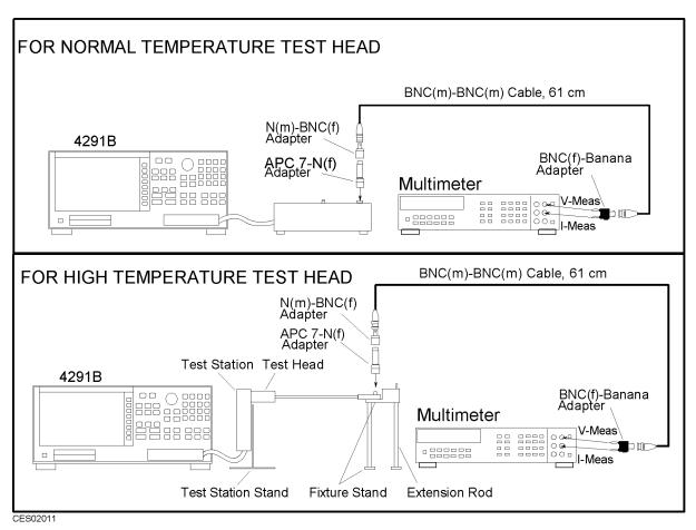
Figure 2-7. DC Bias Level Accuracy Test Setup
