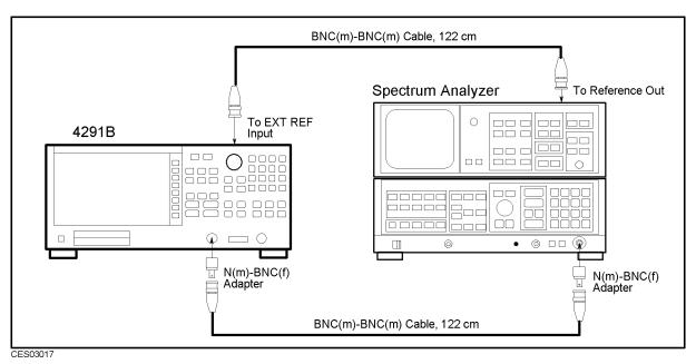
Figure 3-13. Source Mixer Local Leakage Adjustment Setup
