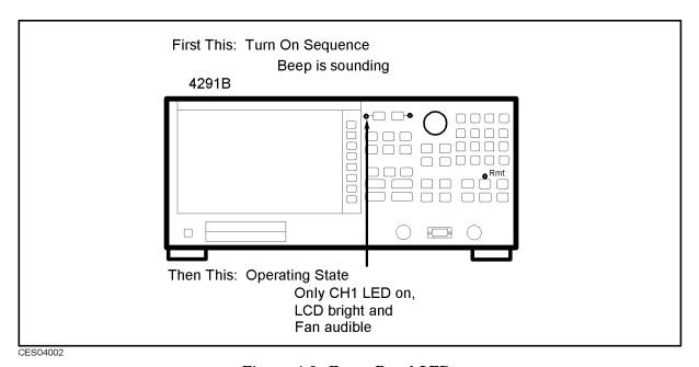
Figure 4-2. Front Panel LEDs
