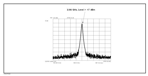
Figure 7-20. Typical 2nd Local Oscillator Signal
