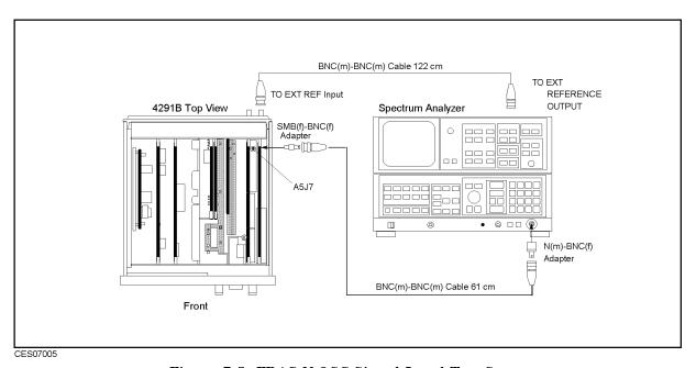
Figure 7-5. FRAC N OSC Signal Level Test Setup
