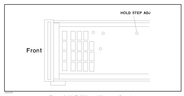
Figure 3-16. Hold Step Adjustment Location
