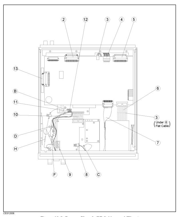
Figure 12-5. Bottom View 2 (RF Cables, and Wires)
