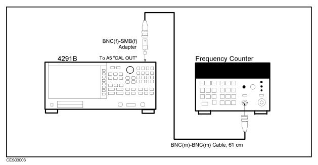
Figure 3-2. 40 MHz Reference Oscillator Frequency Adjustment Setup
