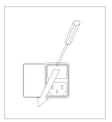
Open the cover of AC line receptacle on the rear panel using a small minus screwdriver.
