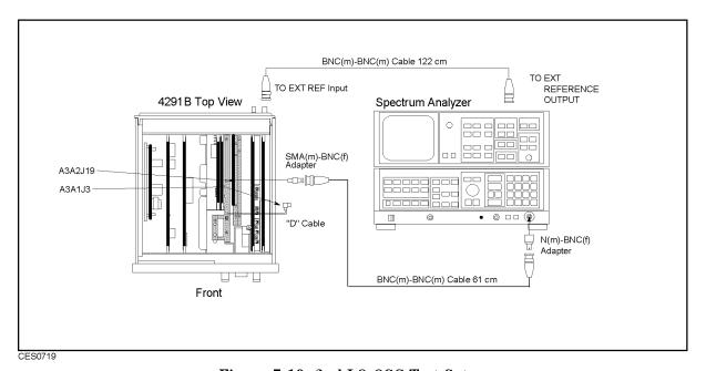
Figure 7-19. 2nd LO OSC Test Setup
