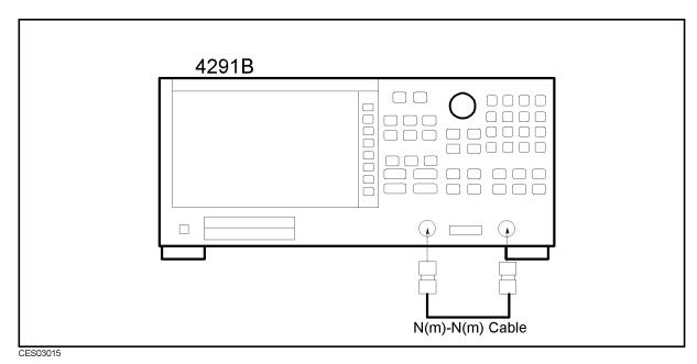
Figure 3-17. Band Pass Filter Adjustment Setup
