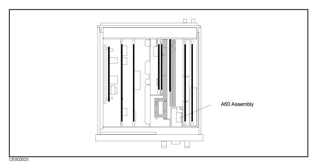
Figure 3-20. 10 MHz Reference Oscillator Frequency Adjustment Location
