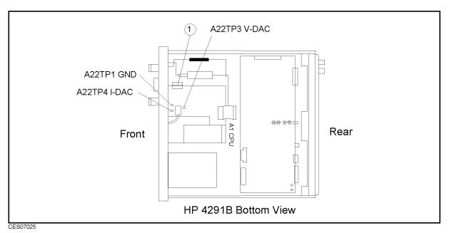
Figure 7-25. A22 Output Voltages Check Location
