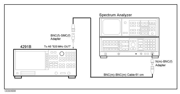
Figure 3-5. 520 MHz Level Adjustment Setup
