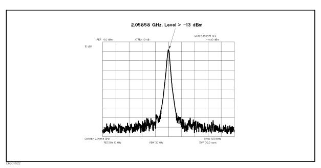
Figure 7-22. Typical 2.05858 GHz Signal
