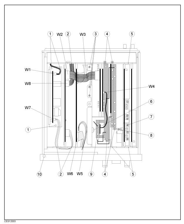
Figure 12-3. Top View 3 (Wires and Misc. Parts)
