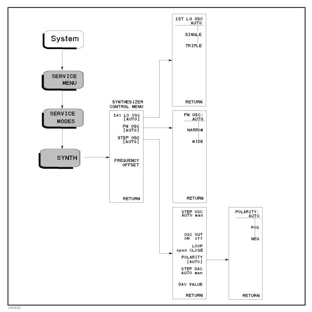
Figure 10-12. Synthesizer Control Menu
