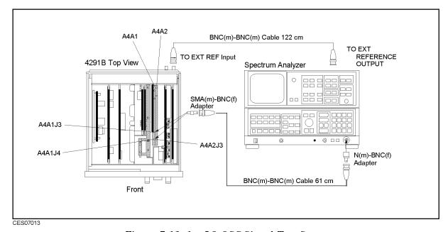
Figure 7-13. 1st LO OSC Signal Test Setup
