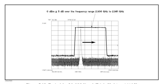
Figure 7-15. Typical 1st LO OSC Signal (Triple Mode) at A4A1J3
