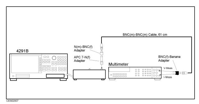
Figure 3-19. DC Bias Level Correction Constants Setup
