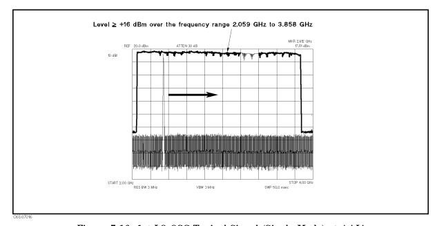
Figure 7-16. 1st LO OSC Typical Signal (Single Mode) at A4J4
