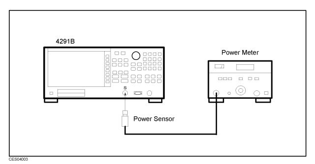
Figure 4-3. Source Test Setup
