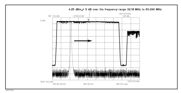
Figure 7-6. FRAC N OSC Typical Signal
