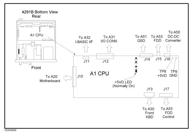
Figure 5-8. A1 CPU Connector Locations
