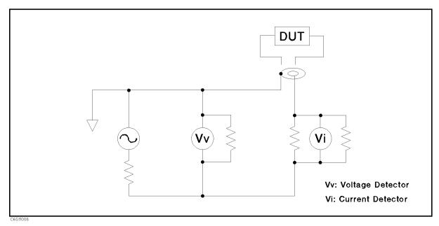
Figure 11-8. High Impedance Measurement Block Diagram
