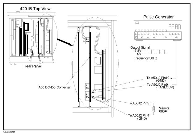
Figure 5-10. A50 DC-DC Converter Troubleshooting Setup
