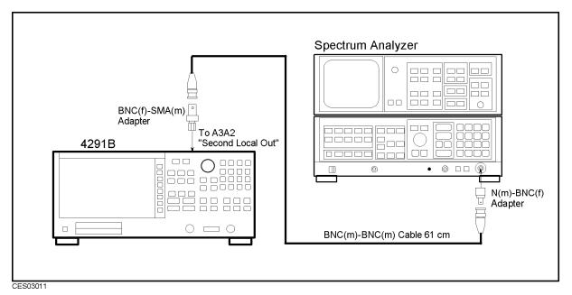
Figure 3-10. Second Local PLL Adjustment Setup
