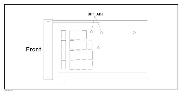
Figure 3-18. Band Pass Filter Adjustment Location
