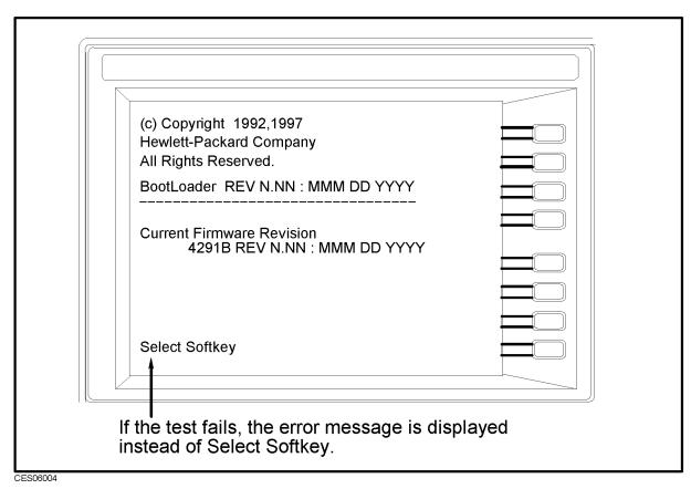
Figure 6-3. Bootloader Display
