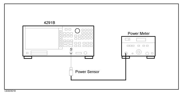
Figure 3-15. OSC Level Correction Constants Setup
