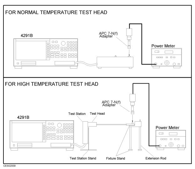
Figure 2-2. OSC Level Accuracy Test Setup
