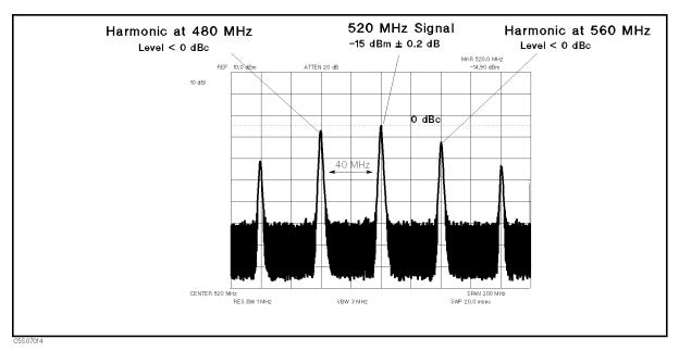
Figure 7-9. Typical 520 MHz Signal
