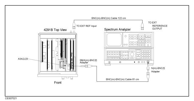
Figure 7-21. 2.05858 GHz Signal Test Setup
