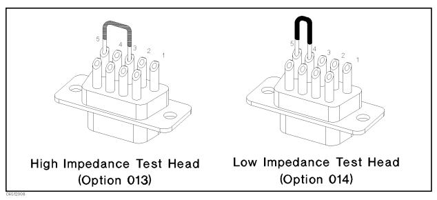
Figure 12-18. ID Connector Wiring
