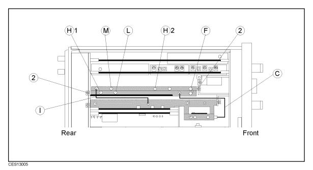
Figure 13-5. A4 First Lo/Receiver RF Replacement
