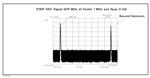
Figure 7-8. Typical STEP OSC Signal at Center 1 MHz
