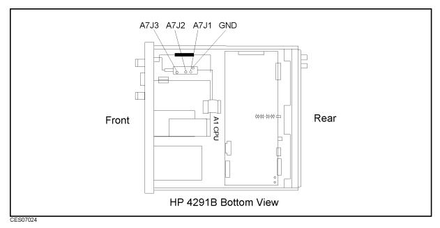
Figure 7-24. A7 Output Attenuator Control Signals
