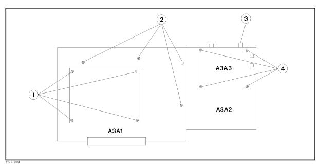
Figure 13-4. A3A1, A3A2, and A3A3 Replacement
