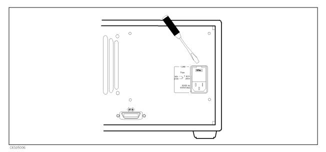
Figure 5-6. Removing Line Fuse
