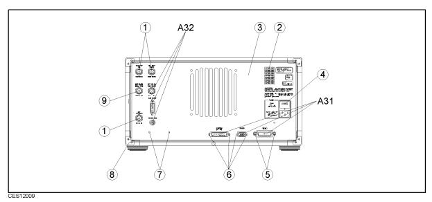
Figure 12-12. Rear Assembly Parts 1 (Outside)
