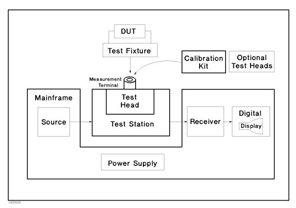
Figure 11-1. Analyzer Simplified Block Diagram
