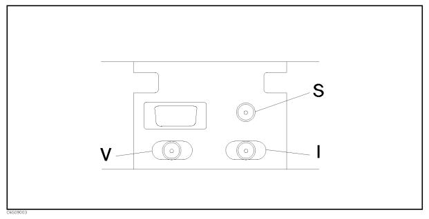
Figure 9-4. Test Station Connectors Locations
