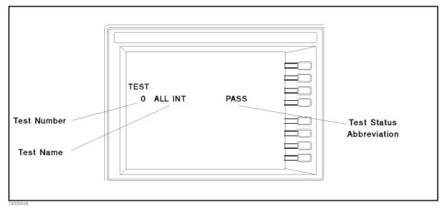
Figure 10-4. Test Status on the Display
