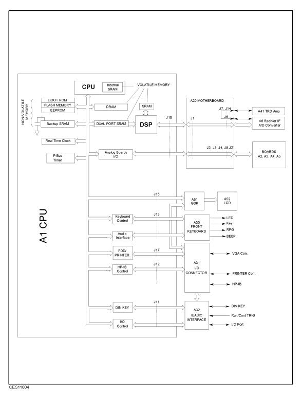
Figure 6-1. Digital Control Group Simplified Block Diagram
