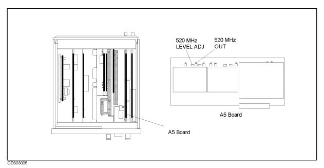
Figure 3-4. 520 MHz Level Adjustment Location
