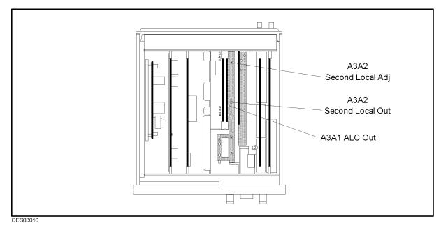
Figure 3-9. Second Local PLL Adjustment Location
