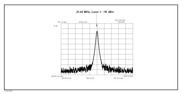
Figure 7-18. Typical 21.42 MHz Signal
