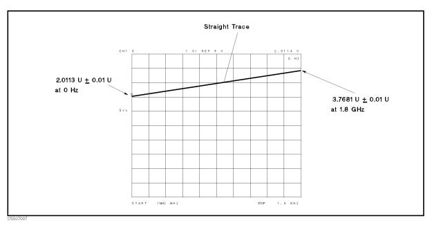
Figure 7-4. Typical FRAC N OSC Signal in Frequency Bus Measurement
