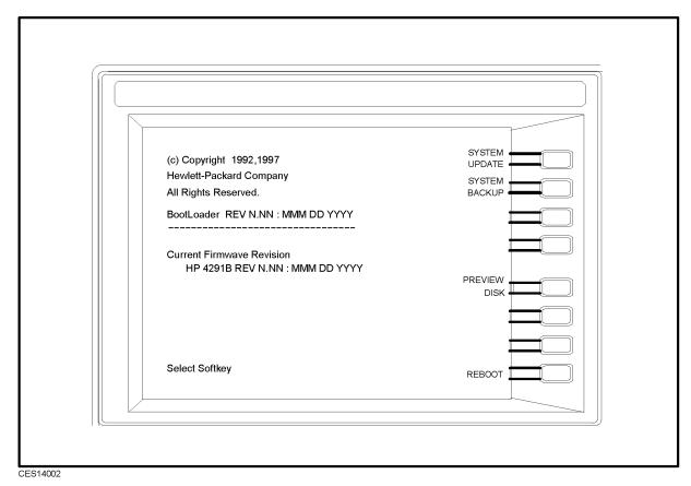
Figure 14-2. Bootloader Menu Display
