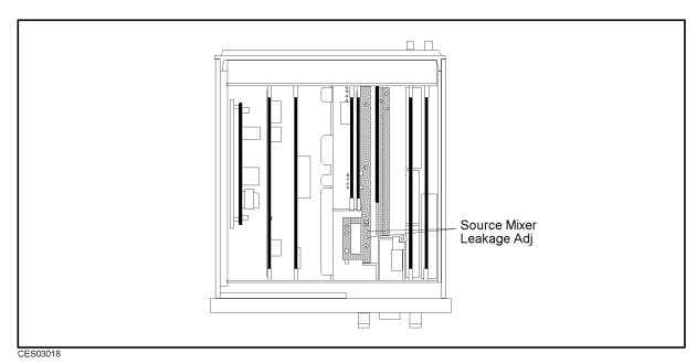
Figure 3-14. Source Mixer Leakage Adjustment Location
