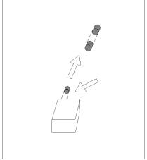
To check or replace the fuse, pull the fuse holder and remove the fuse. To reinstall the fuse, insert a fuse with the proper rating into the fuse holder.
