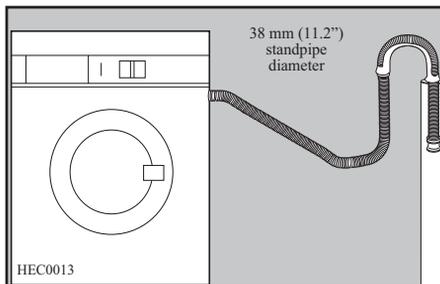
When discharging into a standpipe ensure that the top of the standpipe is no more than 90 cm (35.4") and no less than 60 cm (23.6") above floor level.
