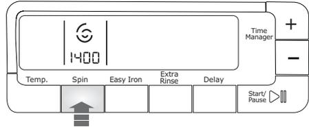
Press the Spin button repeatedly to change the spin speed, if you want your laundry to be spun at a speed different from the one proposed by the washing machine.
