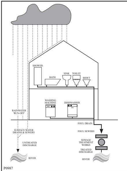
Washing machines and dishwashers should be connected to the FOUL drainage system, the water will then be taken to a sewage works for treatment before being discharged safely into a river.
