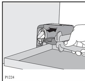
Always keep a rag nearby to dry up spillage of water when removing the cover.
