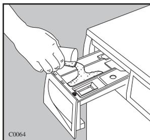
If required, pour fabric softener into the compartment marked
