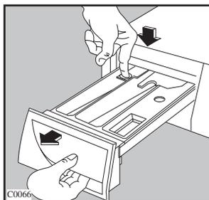
To aid cleaning, the top part of the additive compartment should be removed.
