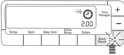
To start the selected programme, press the Start/Pause button; the green pilot light stops flashing.
