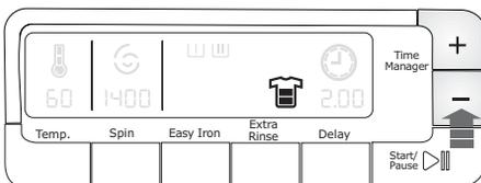
This function allows you to modify the washing time, automatically proposed by the washing machine. By pressing the «**Time manager** buttons «+/-» repeatedly, the duration of the washing cycle can be increased or decreased.
