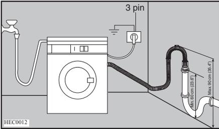
An additional drain hose and joining piece is available from your local Service Force Centre. The joining piece must have an internal diameter of 18 mm.
