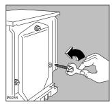
Using a spanner, unscrew and remove the rear right-hand bolt and lay the machine on its back, taking care not to squash the hoses. This can be avoided by placing one of the corner packing pieces between the machine and the floor.
