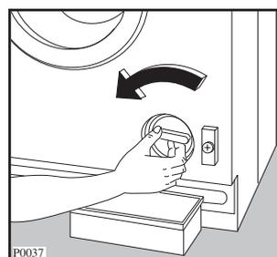
Unscrew and remove the filter.
