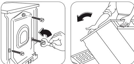
1. Unscrew and remove the three rear screws by means of a key.
