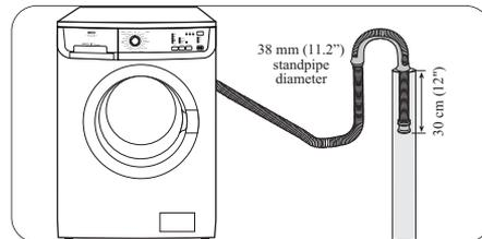
Firstly form a hook in the end of the drain hose using the «U» piece supplied. Place the drain hose into your standpipe, which should have an internal diameter of approximately 38mm thus ensuring there is an air break between the drain hose and standpipe. When discharging into a standpipe ensure that the top of the standpipe is no more than 90 cm (35.4") and no less than 60 cm (23.6") above floor level.
