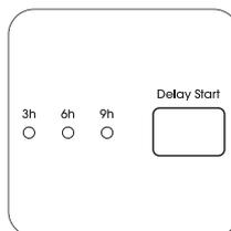
Before you start the programme, if you wish to delay the start, press the Delay Start button repeatedly, to select the desired delay.
