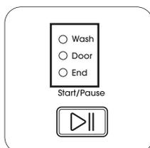
The «Wash» and «Door» lights are alight to indicate that the appliance starts operating and the door is locked.
