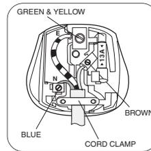
The wire coloured green and yellow must be connected to the terminal marked with the letter «E» or by the earth symbol  $\equiv$  or coloured green and yellow.
