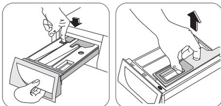
To aid cleaning, the top part of the additive compartment should be removed. Remove the drawer by pressing the catch downwards and by pulling it out. Flush it out under a tap, to remove any traces of accumulated powder.
