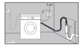
The drain hose may be extended to a maximum of 4 metres. An additional drain hose and joining piece is available from your local Service Force Centre. The joining piece must have an internal diameter of 18mm.
