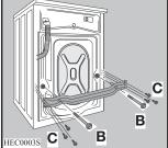
• Remove the bracket **D** and tighten up the six smaller bolts **C**.
