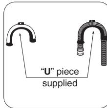
Firstly form a hook in the end of the drain hose using the «U» piece supplied.
