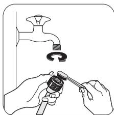
Turn off the water tap. Unscrew the water inlet hose. Clean the filter using a hard bristle brush. Tighten up the inlet hose.
