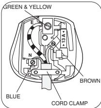
The wire coloured green and yellow must be connected to the terminal marked with the letter «E» or by the earth symbol  $\equiv$  or
