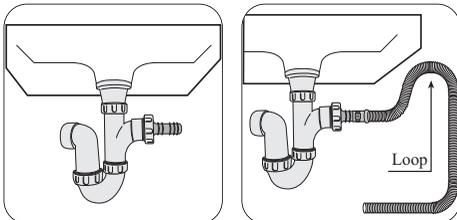
Push the drain hose onto the spigot and secure with a clip, ensure a loop is formed in the drain hose (see diagram) to prevent waste from the sink entering the washer-dryer.
