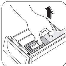
To aid cleaning, the top part of the additive compartment should be removed. Remove the drawer by pressing the catch downwards and by pulling it out. Flush it out under a tap, to remove any traces of accumulated powder.
