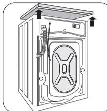
If the counter is too low and it becomes necessary to remove the top lid of the washer-dryer, a steel plate, known as a height reduction kit, must be used.
