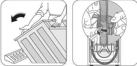
1. After removing all the packaging, carefully lay machine on it's back to remove the polystyrene base from the bottom.
