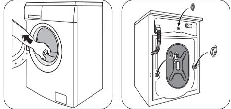
5. Open the porthole and remove the polystyrene block fitted on the door seal.
