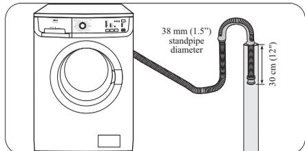
When discharging into a standpipe ensure that the top of the standpipe is no more than 90 cm (35.4") and no less than 60 cm (23.6") above floor level.
