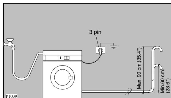
Make sure that it is designed in such a way, that the end of the drain hose cannot be covered with water. The drain hose may be extended to a maximum of 4 metres. An additional drain hose and joining piece is available from your local Service Force Centre. The joining piece must have an internal diameter of 18mm.
