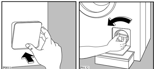
Unscrew and remove the filter.
