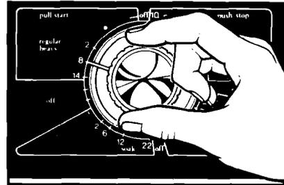
**B.** Stop on a number in the cycle you want. The numbers are minutes of wash time. The drawing shows 8 minutes of agitation in the REGULAR HEAVY Cycle.
