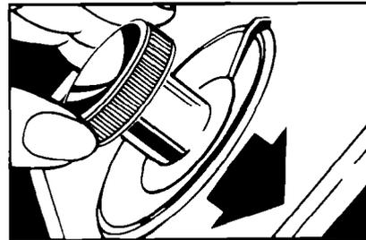
**D.** To stop the washer at any time push in the Control Knob. To restart the washer, pull out the Control Knob. To set the controls for a rinse and spin, a drain and spin, or a soak or pre-wash, see page 8.
