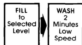
**\*NOTE:** THE WASHER WILL PAUSE BRIEFLY THROUGHOUT EACH CYCLE. These pauses are normal. They allow for the reversing of the motor, normal washer operations, and the cool down portion of the PERMANENT PRESS Cycle
