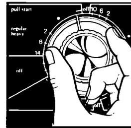
3. Set the washer for a DRAIN and SPIN (see page 8). Let it run for about 30 seconds to mix the antifreeze and water.
