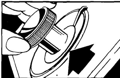
**C.** Start the washer by pulling out the Control Knob. The washer will fill to the level you set with wash water of the selected temperature. After filling, the washer will agitate for the selected number of minutes.
