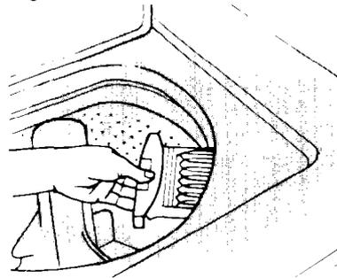
To remove it for cleaning, press the release and pull straight out. Instructions for cleaning are printed on the bottom of the filter.
