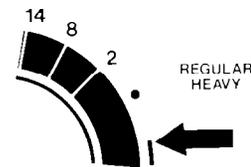
The washer will drain, spin out water and stop. If you want a low-speed spin, use the bar on PERMANENT PRESS or KNITS GENTLE. All the other cycle settings have a high-speed spin.
