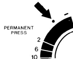
There is a dot just after the numbers in PERMANENT PRESS, REGULAR HEAVY and KNITS GENTLE. If you push in on the Cycle Control Knob, turn the pointer to one of those dots and pull the Control Knob out, the washer will fill, agitate, drain and spin.
