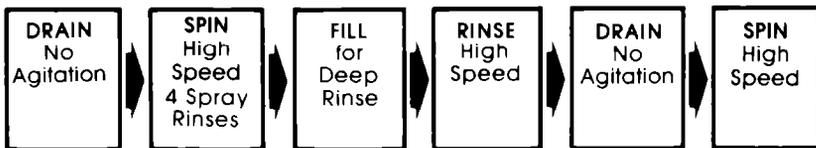
\* **IMPORTANT: THE WASHER WILL PAUSE BRIEFLY THROUGHOUT EACH CYCLE. These pauses are normal. They allow for the reversing of the motor, normal washer operations, and the cool down portion of the PERMANENT PRESS Cycle.**
