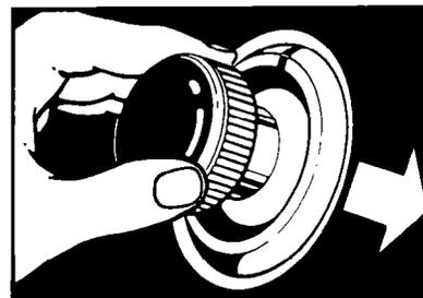
**D.** To stop the washer at any time, push in the Control Knob. To restart the washer, pull out the Control Knob.
