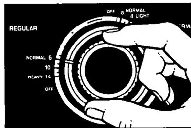
**B.** Stop on a number in the cycle you want. The numbers are minutes of wash time. The drawing shows 6 minutes of agitation in the REGULAR NORMAL Cycle.
