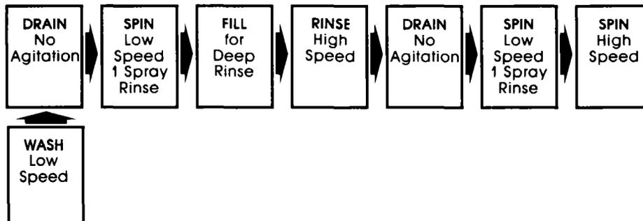
**\*IMPORTANT: THE WASHER WILL PAUSE BRIEFLY THROUGHOUT EACH CYCLE. These pauses are normal. They allow for the reversing of the motor, normal washer operation, and the cool-down portion of the PERMANENT PRESS Cycle.**
