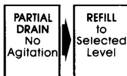
The washer will proceed to the REGULAR/HEAVY Cycle. If you want a different cycle to follow SUPER WASH, push in the cycle control knob, turn to the cycle and time you want, pull knob out to start.
