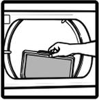
2. Roll lint off the screen with your fingers. Do not rinse or wash the screen to remove lint. Wet lint is hard to remove.
