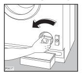
Unscrew and remove the filter.
