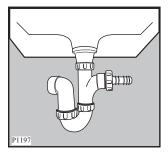
Push the drain hose onto the spigot and secure with a clip if required, ensure a loop is formed in the drain hose (see diagram) to prevent waste from the sink entering the washer dryer.
