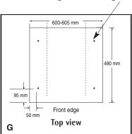
Position the base into the recess with its front edge as far forward as the adjoining plinth line will allow.
