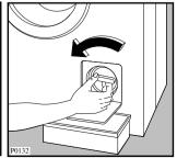
Unscrew and remove the filter.
