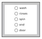
After the machine has started, only the running phase pilot light stays on.
