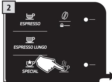
Press the hot water button and wait for the dispensing of the programmed water quantity. Water dispensing can be interrupted at any time by pressing "STOP HOT WATER".
