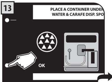
Place a container under the dispensing spout and a container under the hot water wand.
