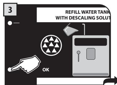
Refill water tank with descaling solution.
