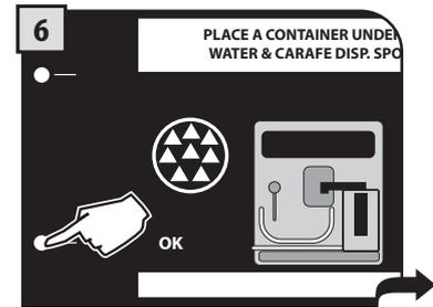
Place a container under the dispensing spout and a container under the hot water wand. Then, press the "OK" button.
