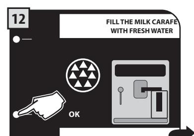
Completely empty the carafe (page 38 - fig. 7) and fill it with fresh water. Insert the carafe in the brewing position, and then press the "OK" button.
