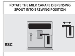
A beverage with milk has been selected. The machine requires the carafe handle spout to be placed into dispensing position.
