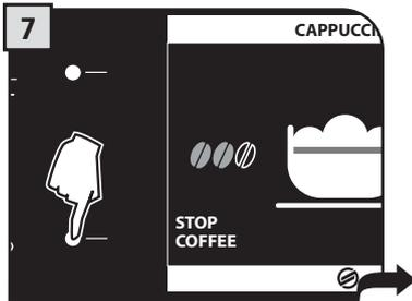
Once milk has been dispensed, the machine starts brewing the coffee. Coffee brewing can be interrupted at any time by pressing "STOP COFFEE".
