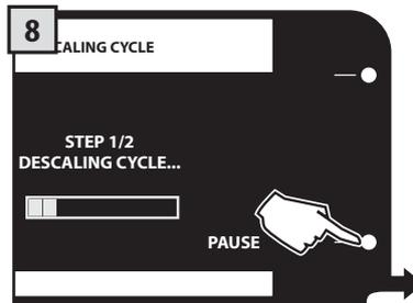
If the containers need to be emptied, press the "PAUSE" button. Then, press the "START" button when the container has been emptied and replaced.
