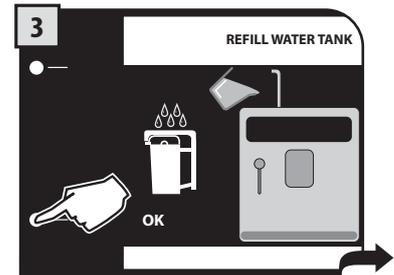
Fill the water tank with fresh drinking water. Press the "OK" button to confirm.
