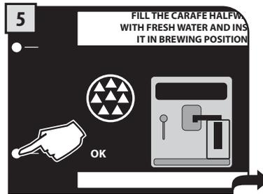
Fill half the carafe with fresh water (page 38 - fig. 7). Insert the carafe and place it in the brewing position. Then, press the "OK" button.
