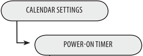
This menu allows you to programme the machine power-on times, according to your needs. The machine performs this function only if the power button is switched to on.
