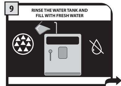
At the end of the first step, when the descaling solution is finished, the machine will require a tank rinse.
