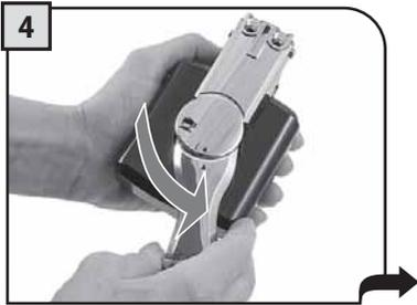
4 Rotate the handle counter-clockwise to the unlock position.
