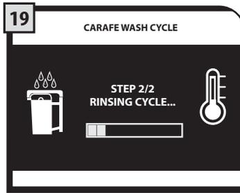
The rinse cycle is activated. The bar shows the cycle progress. At the end of the cycle, the machine returns to the product brew menu page.
