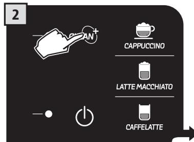
Press the cleaning cycle button. The machine executes an additional cleaning cycle.
