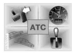
On vehicles with an automatic transmission, the Adaptive Transmission Control (ATC) uses a number of factors to calculate the gear which provides maximum efficiency. In this process, it considers your individual driving style as well as current driving conditions.
