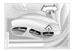
3 Backrest angle Pull the lever and apply weight to or remove weight from the backrest to reach the desired position
