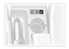
Use this button to operate the central locking system when the front doors are closed. The doors and tailgate are unlocked or locked only. The anti-theft alarm system is not activated.
