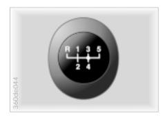
Completely depress the clutch pedal each time you shift, pressing the manual-shift gear lever into its respective end position.
