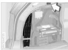
The hazard warning triangle is stored on the left-hand side of the luggage compartment behind the cover panel. To open: press the button (arrow) and remove the cover.
