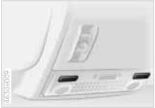
In order to prevent draining the battery, all of the lamps in the vehicle are switched off automatically approx. 15 minutes after the ignition key is turned to position 0. ◀
