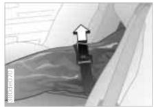
Secure the skis or other objects in the bag by tightening the strap with the buckle.
