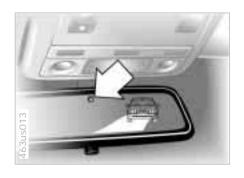
The semisolid reacts chemically to this electrical current, thus providing dimming of the mirror through an infinitely-variable range (electrochromic technology).
