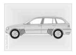
There is an antenna located right near every wheel in the vehicle body. This antenna picks up signals from its respective wheel. A central electronics system evaluates the quadruple signals which it receives and forwards any changes.
