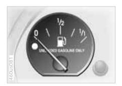
When you switch on the ignition, the indicator lamp lights up briefly as a function check.
