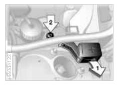
cover of the auxiliary terminal for jump-starting is identified by a "+" sign. Refer to the illustration. Remove the cover by pulling the tab (arrow 1).
