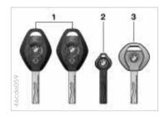
1 The master keys with remote control determine the functions for the Key Memory; refer to page 52
