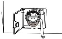
4. Open the pump by turning its cover anticlockwise. Lift off the cover and coin trap.
