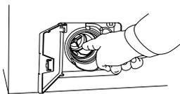
5. Clean out any objects and foreign matter from the pump housing. Ensure that the pump blade, at the rear, can be rotated.
