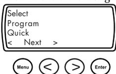
3. If you wish to change a setting, you should index forward or back with the **<** **>** buttons until the desired setting appears in the display.
