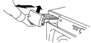
Flush and brush the detergent compartment to remove any residues.
