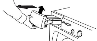
Flush and brush the detergent compartment. Put the detergent compartment back in.
