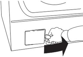
3. Drain off the water, eg, in a bowl, by pulling loose the drain hose from its connection on the inside of the cover.
