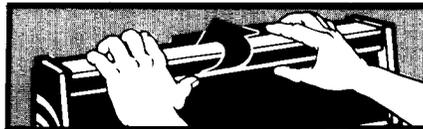
1. Flip up the console top by grasping it with both hands near each end and lifting the front edge up.
