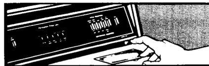
The fluorescent console light is under the console top. The **Console Light** switch is on the bottom right side of the console. To turn on the light, push in the switch and hold it for a second or two. Push the switch again to turn the light off.
