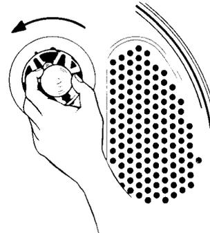
3. Replace the bulb with a 40-watt appliance bulb only.
