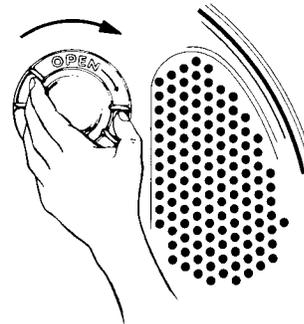
2. Remove the light bulb by turning it counterclockwise.
