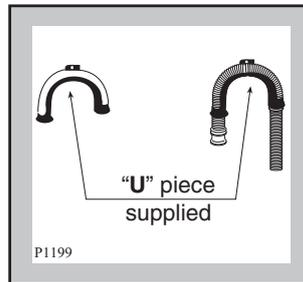
lace the drain hose into your standpipe, which should have an internal diameter of approximately 38mm thus ensuring there is an air break between the drain hose and standpipe.
